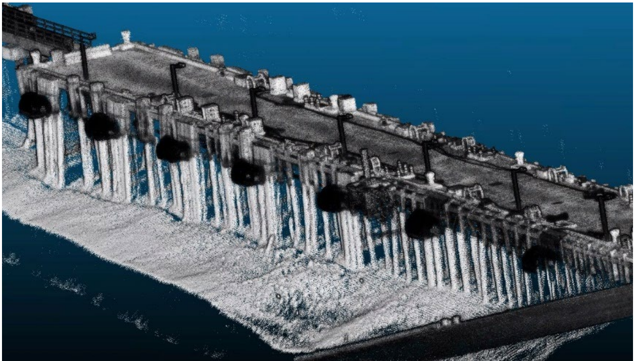
Image N213-140-3: 3D sonar and LiDAR point cloud data of typical pier in typical usable condition. This image vaguely illustrates how tough it is to obtain under-pier data via motoring around the perimeter of a structure.
